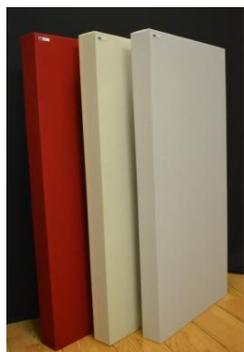
The **242 Acoustic Panel** measures 24.25" x 48.5" x 3.5" and has a built-in air gap which not only increases low end absorption, but allows the panel to hang truly flush on the wall. Perfect for first reflection points or above the listening spot.
