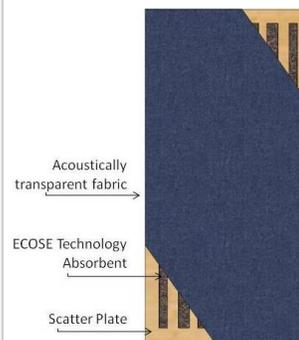
GIK Acoustics offers the built-in **Scatter Plate** option – a wooden plate that adds one-dimensional scattering / diffusion. The **Scatter Plate** is built-in between the fabric and the absorption material on GIK's 242 Acoustic Panel, 244 Bass Trap, Monster Bass Trap, Tri-Trap or ArtPanel.
