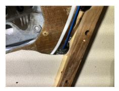
The nav pod was being installed in the same location as the previous instrument pod for the old ST50 instruments. However, I had to grind out and make the holes bigger in the pedestal guard to accommodate the SeaTalkNG connectors.
