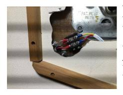
The 14 AWG 2-wire safety marine cable was run aft from the 6-way junction block aft through the same conduit as the back bone cable for the network. Once in the lazarette, it was led aft through the same black conduit running aft of the lazarette to the centerline and then up and into a 2-way junction block at the bottom of the helm pedestal. The wiring (R70523) from the Axiom +9 was run down through the port pedestal guard into the 2-way junction block to make the connection.
