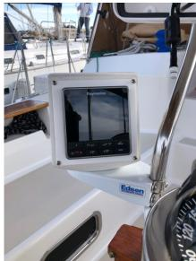
Prior to installing the I70s in the nav pod, resistance checks were done on the back bone cable to ensure there was 60 ohms. The resistance check between Can A and Can B on the I70s spur cable read 59.9 ohms.
