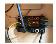
I removed the blue terminator plug and unplugged the power from the backbone in order to continue with the installation.
