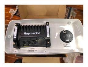
Axiom +9 was connected to the back bone using the provided SeaTalkNG to DeviceNet adaptor cable.
