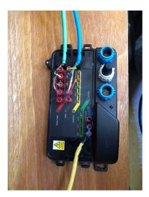
connector and cut wire. Strip back 0.5 in, twist and bend back for 0.25 in that is inserted in the next female spade connector and crimp. Continue the process with the white wire and then the brown wire. Position shrink wrap and heat. Perform the exact same process for wind (I used blue shrink wrap). For depth, because there are only 3 wires instead of five, I initially
