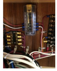
At this point, with the EV-1, iTC-5 converter with depth, speed and wind installed, the 5-way back bone connector, and I70s installed; a systems check was warranted to test the installation
