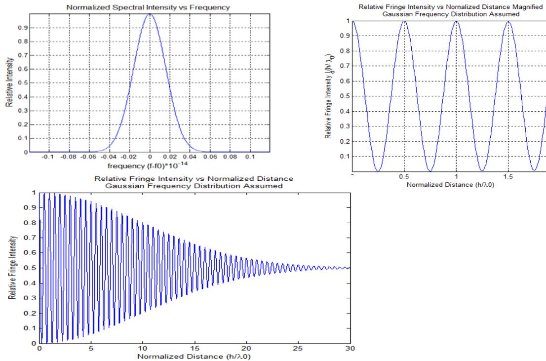
**Figure 2. LED Spectrum Light and Michelson Interferometer Fringes**
