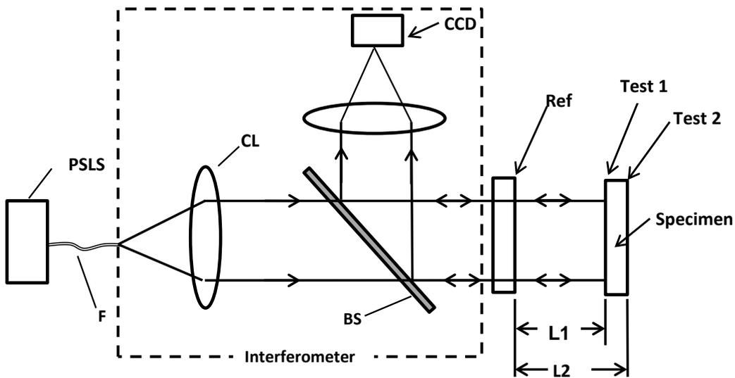
Figure 4. Fizeau Interferometer Schematic with Phase-Shifted Light Source
