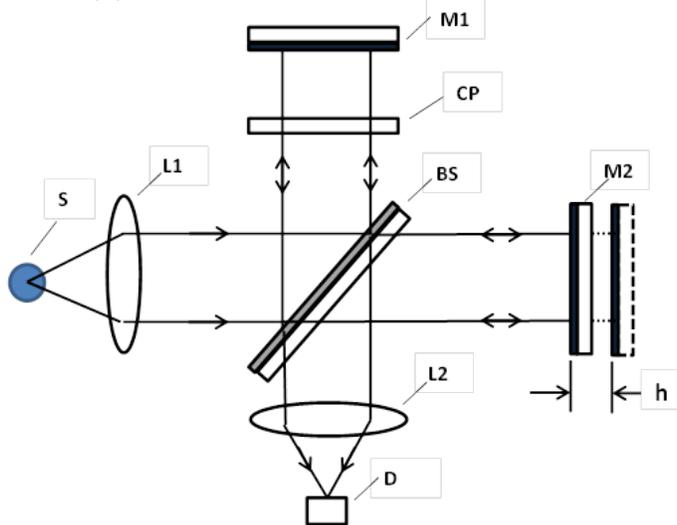
Fig. 1. Schematic of Michelson Interferometer with Broadband Source
