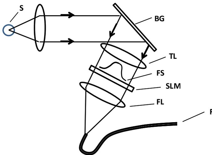
**Fig. 3. Illustrative Schematic for Phase-Shifted Broadband Light Source**
