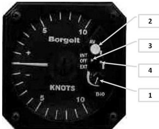
The Borgelt B40 variometer provides total energy rate of climb displayed on the round meter with accompanying audio.
