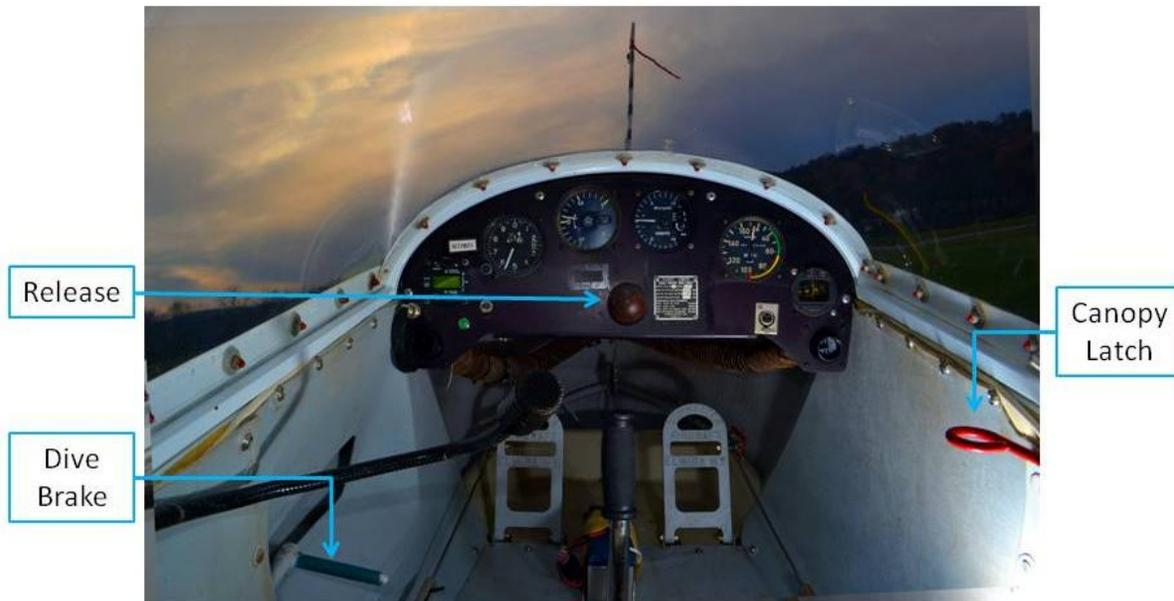
*Figure 2 SGS 2-33A Front Cockpit*
