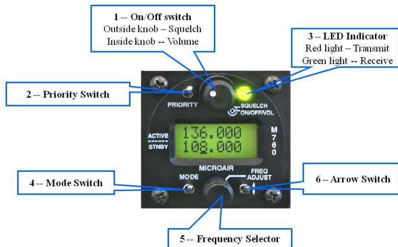
*Figure 1 MicroAir Radio*
