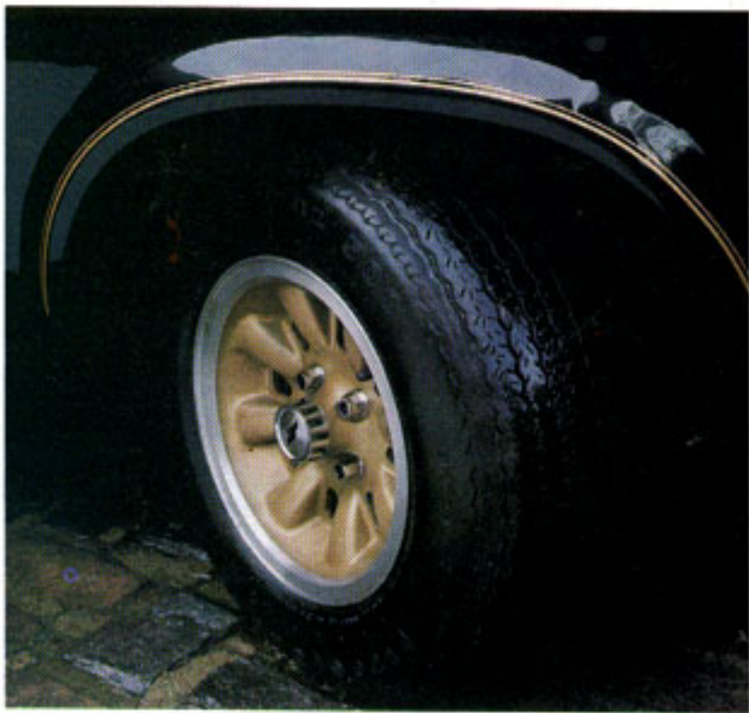
Cast aluminum alloy wheels and radial ply tires.
