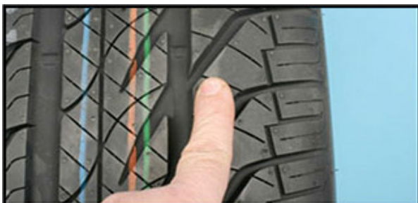
Angled grooves, referred to as lateral grooves, direct water out from the longitudinal grooves to aid in water evacuation. Water is collected in the main grooves and directed out of the tread area via lateral grooves.
