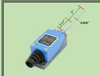
The limit switch selected is a model TZ-8169, a SPDT switch that has a thin, 0.050 inch diameter, 2 inch long probe wound into a spring that is 1 ¼ inches long before entering the switch. It has both normally closed and normally open terminals. The device only uses the normally open contacts which close if the probe is touched by a mirror.
