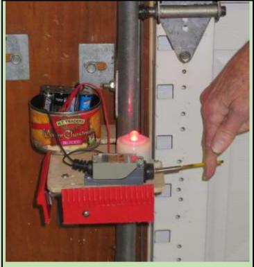
When the limit switch is pressed the alarm and flashing light are energized. You can see the light in this photo. If the warbling sound doesn't get your attention the flashing red light will-especially at night. Frankly nighttime is when the extra precaution may come in handy for that once in a thousand occurrence as I get more complacent about pulling the C7 out of the garage! The \$20 cost is 30 times less than a mirror repair!
