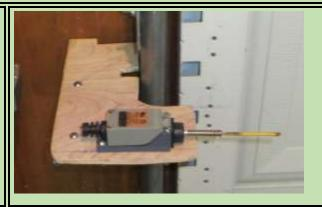
A 100 dB, 12 volt alarm, with a flashing red indicator light, was purchased on ebay for under \$7. The sound is a warble and is readily heard over any engine noise. A quick look to the right while pulling out of the garage will also show a flashing light if getting too close to the edge. The probe remains activated as it bends and until any force is removed.
