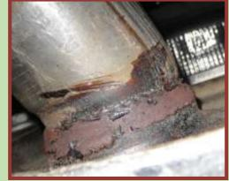
the brown rust to a dull black finish with rust reformer. It also helps reduce further oxidation.
