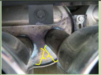
This picture was taken after a few brush strokes were made over the rusted area. Two areas are marked in yellow. The milk like, somewhat foamy reformer looks light blue in this picture as well as the one below. It is best to put on some light coats than come back and repeat in a few minutes.
