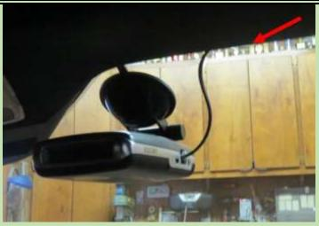
Mounting the detector high on the windshield to the right of the mirror eliminates any obstruction to road vision. However routing the wire so it is not visible, is a challenge. The first area was across the top of the windshield. It was not possible to insert the wire behind the top window trim so a piece of rubber "D" shaped hollow molding (that we use in our business) provided a good solution to hide this section of wire.
