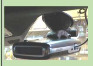
Several months after the 1<sup>st</sup> failure, on a hot day in SC, the car was parked for 1 hour in the sun, found the detector hanging from the tether! Glad I added it!
