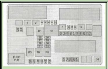
Removing the mini fuses requires a tool. There is one included in the fuse panel. It is shown schematically and labeled FUSE PLR (lower left.) Simply select the fuse desired and squeeze it with the tool, then pull upward. In this case there is a 20 amp fuse for the auxiliary power. When the fuse is removed, it is placed in one of the two fuse locations in the Add-A-Circuit device purchased to supply the detector power.
