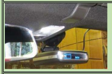
Now the radar detector is energized when the engine starts and is not powered when it is not running. The detector can be easily removed by pressing a simple release if parking for in a questionable area (something I seldom do.)
