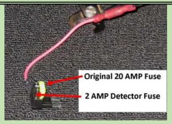
This picture shows an Add-A-Circuit connected to the 12 volt power wire going to the radar detector. Note, the original 20 amp fuse removed from slot # 37, goes in the fuse slots closest to where the device plugs back into the fuse panel. A 2 amp mini fuse is inserted in the other fuse holder. The pigtail wire is seen coming from that fuse. A male/female spade connector is used to connect the wires.
