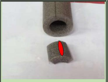
Note: for the similar size section of black, heavy wall heater hose that replaced the soft insulation that took a set and stopped working well, had to put a small groove in the upper section with a round file to have it hold in place. See red area above.
