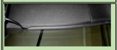
The "D" rubber molding in place under the top widow molding. It is not readily visible even when sitting in the passenger seat. Note some folks have recently said they were able to lift the upper molding, held with clips, and routed the wires under it. They indicate removing the vanity mirror mounts, see my 1<sup>st</sup> pics.
