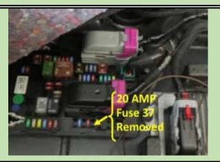
The detector was operating fine with the Smart Cord plugged into the console auxiliary power plug, so why not wire it to that fuse? The C7 has two fuse panels, one in the engine compartment, and one in the rear. The fuse for the auxiliary power, #37, is in the rear, under the rear cargo carpet. Strongly suggest unclipping the bottom of the right wheel cover to allow the carpet to be pulled out from under, or it could rip the corner!
