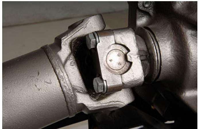
turning the shaft by pushing up or pulling down on the screwdriver. Note any movement in the shaft that would indicate a loose joint.
