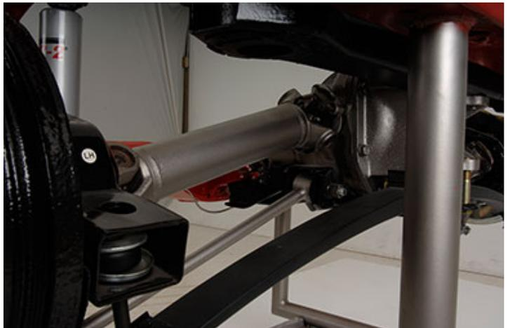
secure the U-Joint into position.
