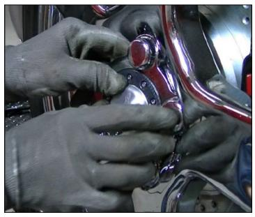
**14.** Put the lug nuts back on the wheel and tighten in a 5 point star pattern to 50 ft/lbs, repeat at 75 ft/lbs, then a final 100 ft/lbs, which is the recommended torque.
