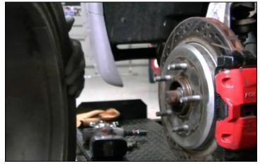
1. Start by removing the Center Cap of the wheel, then loosen and remove the lug nuts.
