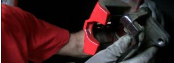
7. Now remove the caliper bracket from the caliper.
