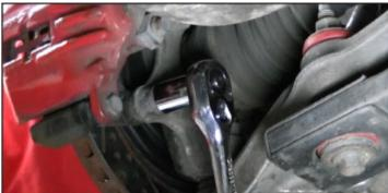
3. Remove the Caliper Bracket Bolts.
