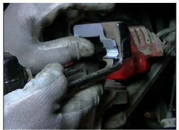
8. Install new brake clips into the bracket.
