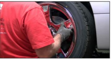
**13.** Use a torque wrench to tighten the caliper bracket bolts to 125 ft/lbs, then put the wheel back on the wheel studs.
