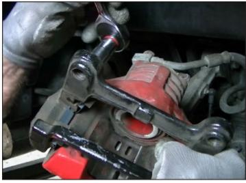
$\textbf{9.} \ \, \text{Once the brake clips are installed, put the bracket back on the brake caliper, tightening to 23 ft/lbs.}$
