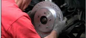
5. Remove the old rotor by pulling it toward you, off of the hub. Next replace it with the new rotor.
