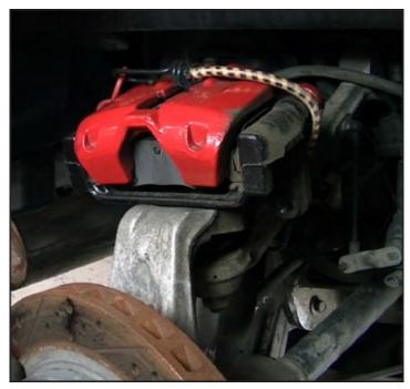
4. Now that the Caliper Bracket Bolts have been removed, you'll want to use the Bungee Cords to strap the caliper in place. ......
