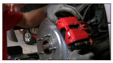
**12.** Using a caliper piston compressor tool (104005), compress the piston and set the caliper back into the original position.
