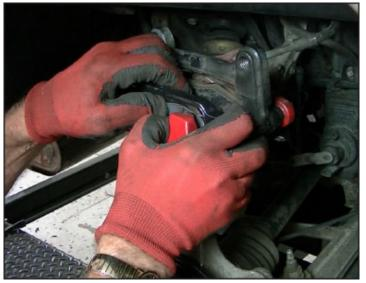
**6.** Once the rotor is installed, you can replace your brake pads. Remove the old pads by popping the brake pads out of the calipers.
