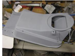
When maintaining the original finish is not a priority, the box can be lightly bead blasted. If the box is cracked or seams are misshapen, *carefully* use heat to soften the material and
