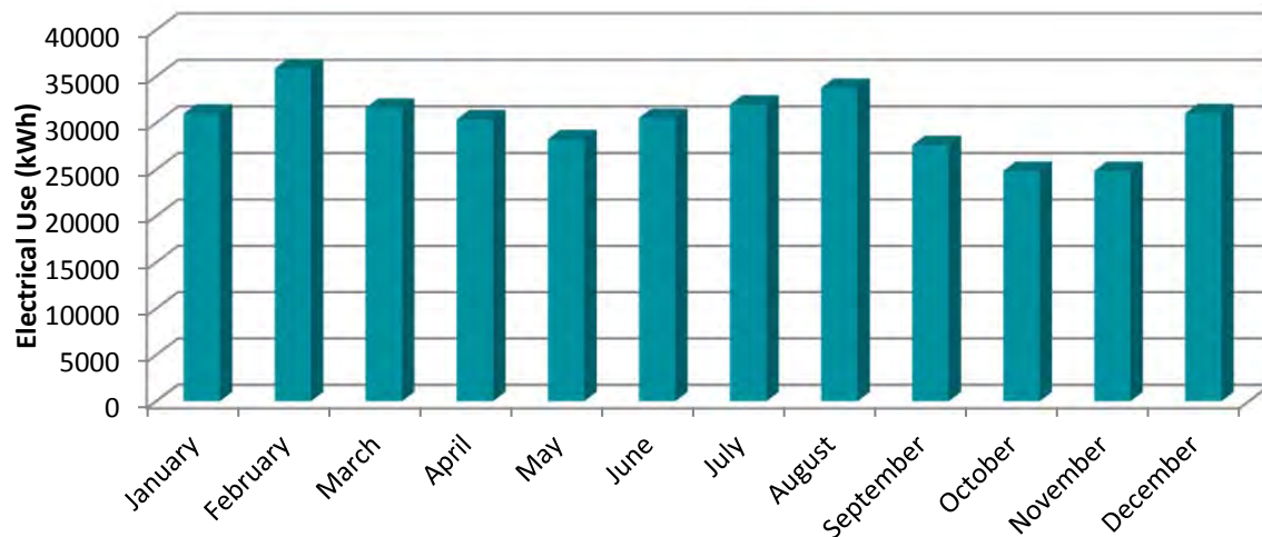
Figure 3.2-1: Administration Building Electricity Usage
