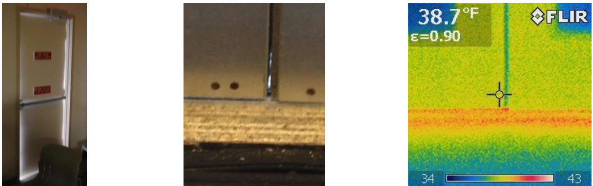
Signs of worn or missing weather stripping at some doors
