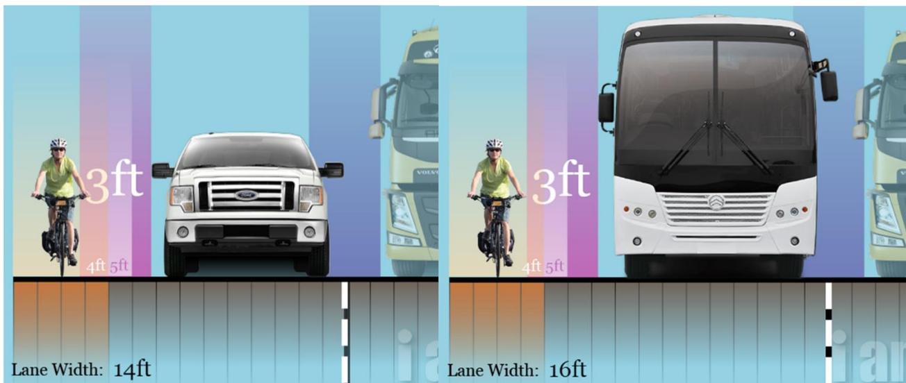
**Above: The minimum pavement width for safe passing of a bicyclist by most cars, SUVs and pickup trucks is 14 feet. The minimum pavement width required for safe passing by a truck, landscaping trailer, or bus is 16 feet. Greater width is required as speeds increase. [Images: see <http://iamtraffic.org/resources/interactive-graphics/> ]**
