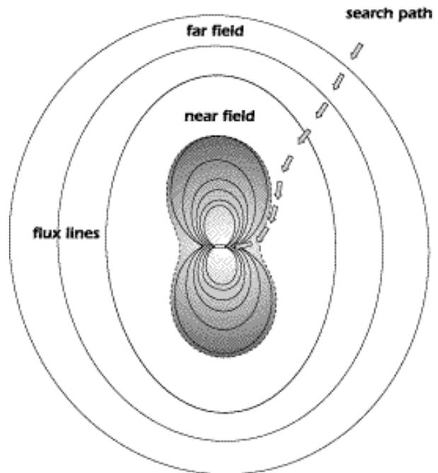
**Near field/ far field.** In the near field, the shape of the signal can be quite complex. A far-field application would point directly to the source.
