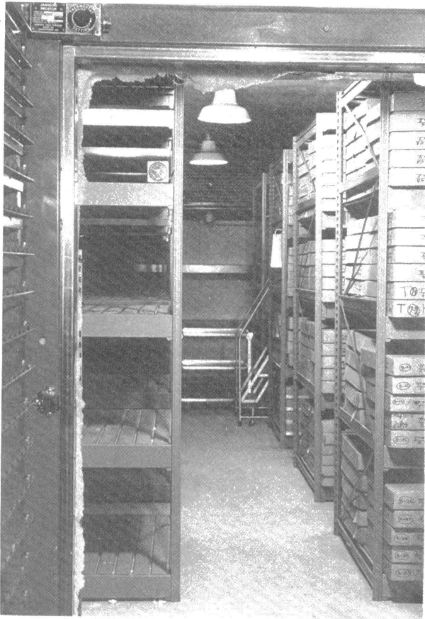
Dry Valley Drilling Project cores stored at -23^{\circ}\text{C} . Rack units are modular and can be reassembled as necessary without the use of connective hardware.
