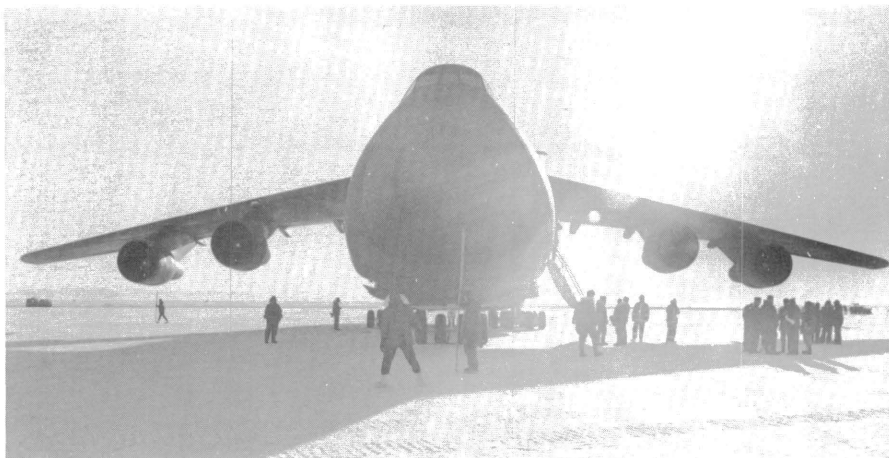
This C-5B Galaxy carried four fully assembled UH-1N helicopters to McMurdo Station from the United States. The helicopters were brought two at a time along with passengers and cargo. Because the helicopters did not have to be disassembled, U.S. Navy helicopter crews from the Antarctic Development Squadron Six were able to begin austral summer operations several weeks earlier than usual. The National Science Foundation, which funds and manages the U.S. Antarctic Program, hopes to continue to use these airplanes to improve operations in Antarctica.
