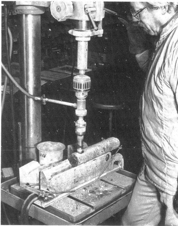
Figure 1. Frozen Dry Valley Drilling Project core segment being dry-drilled for paleomagnetic sample plug by Don Elston, U.S. Geological Survey.
