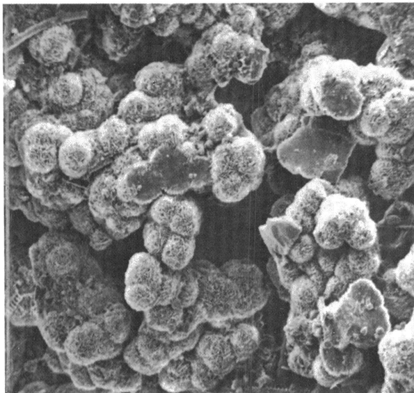
Figure 3. Left: Scanning electron micrograph (enlarged x650) of a fracture surface through a chert pellet recovered from the transition zone in Eltanin core 47-15. The chert is composed of blade-shaped crystals of unidimensionally disordered alpha-cristobalite, arranged in microspherulites about 10 microns in diameter. Right: View at higher magnification (x4,200) of the cristobalitic chert. Shown are thin, tabular crystals which compose the microspherulites, and partially dissolved fragments of siliceous microfossils which constitute the source material of the opaline silica. The arrow points to heavily etched diatom frustule.
