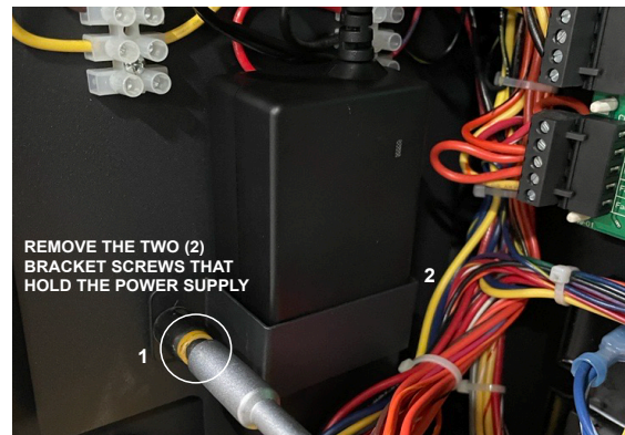
Figure 3. Power Supply Removal
