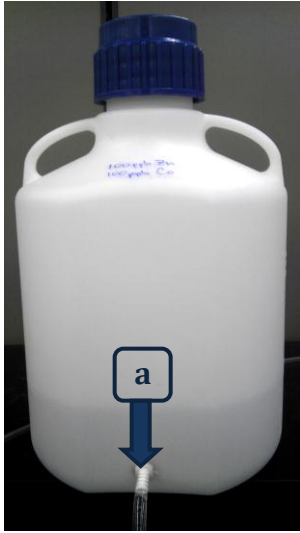
Example of supply vessel with barbed bulkhead fitting
