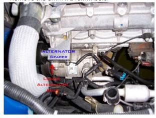
2. Install lower manifold support bracket locating it almost center and low on the motor under the intake using (2) 10mm x 55mm bolts. Tighten to **30 lb/ft** (*See figure* 2)
