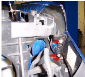
14. Remove the (8) body screws (4 per side) from the bottom of the front bumper cover and the (2) plastic
