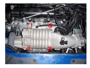
21. Connect the brake booster vacuum line to the hose barb on the blower that points towards the motor.
