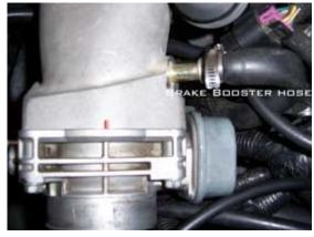
22. Using the 5/16" vacuum line supplied in the kit connect it to EVAP solenoid and the hose barb fitting on the throttle body that faces the radiator support.
