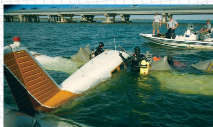
Small aircraft salvage using Enclosed Flotation Bags 2,000 lbs.
