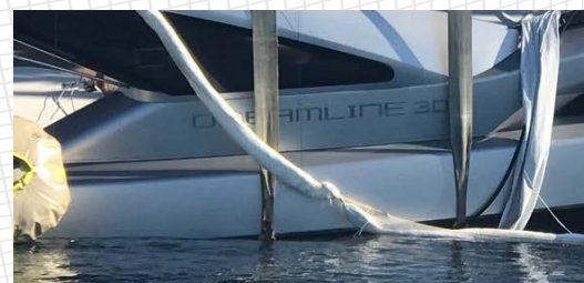
Yacht salvage using Salvage Pontoons 2,000 lbs. and Salvage Pontoons 20,000 lbs. Photo credit: Vessel Assist - San Diego.
