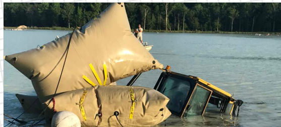
Pulling a CAT out of the lake using Enclosed Flotation Bags 4,000 lbs. and 6,000 lbs. Photo Credit Tow BoatUS Indian River
