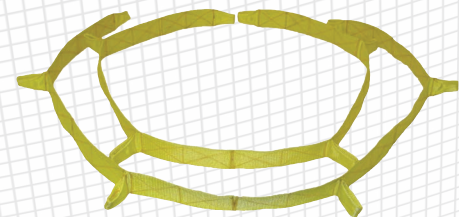
FS10-Flex Straps 4" x 10': • The SUBSALVE Flex strap is 4" by 10' heavy nylon lift strap with 6 lift eyes per strap • 6000lb Safe working load per eye • 2 straps per set
