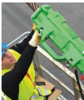
WIRE ROPE CLEANING & LUBRICATION
