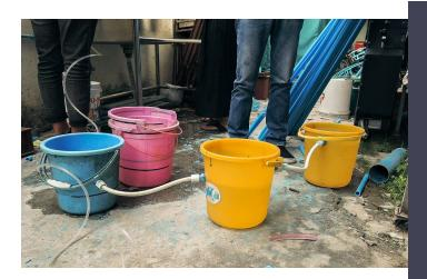
Using plastic buckets as proxies to steel sinks and conducting simple experiments, our team was able to test prototype flow dynamics of the washing station design.
