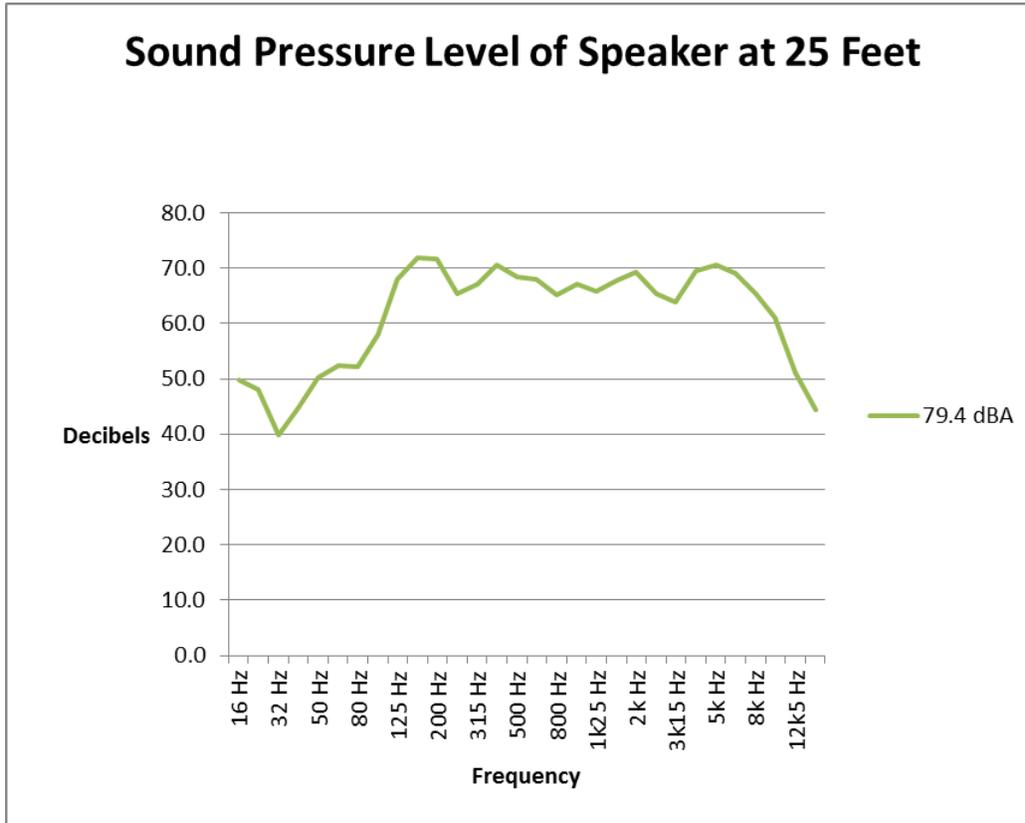
The outside noise level was determined by measuring the sound pressure level (both A-weighted and 1/3 octave band levels) at 25 feet, the same distance the speaker was set up from the façade, but without any obstructions or reflecting surfaces nearby. The speaker and microphone were each between 9 and 10 feet high. The speaker was 79.4 dBA Leq at 25 feet.
