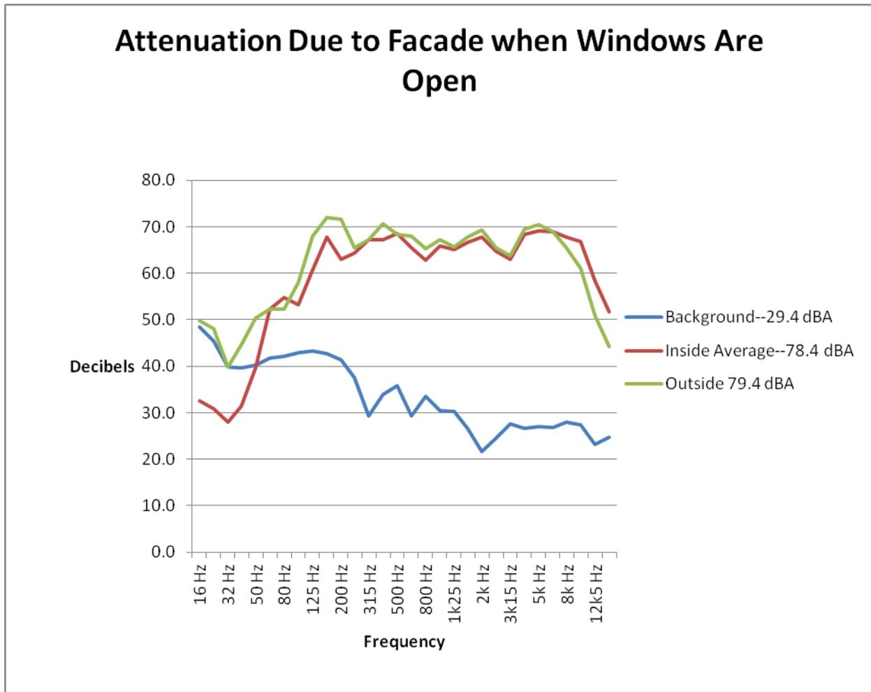
The reduction in noise levels in the important bands between 80 and 5000 hz, is quite small. Overall, there was a 1 dBA reduction in noise levels between outside and inside when windows are open.
