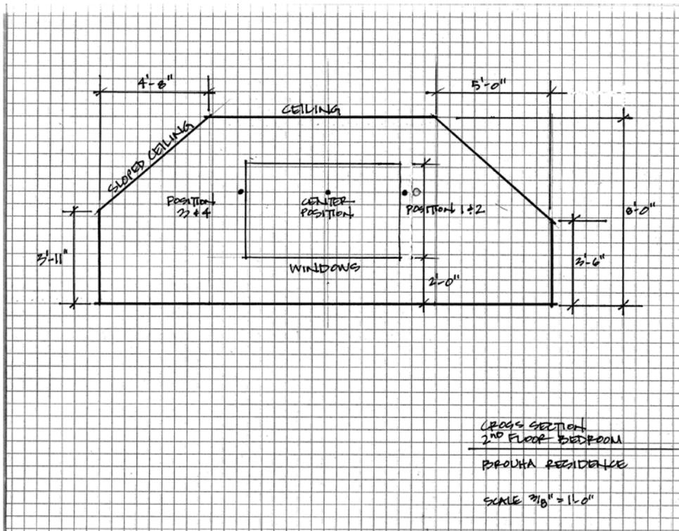
The room volume is 1558 cubic feet. Two beds were removed because they were located where four of the microphone locations were located and to reduce room absorption. The area rug was removed from the room as recommended in the ASTM procedure (at 7.4.1). The following hard objects were left in the room to increase diffusion: 3 plastic storage containers, 3 night stands, 1 desk, 1 small table, 1 luggage frame, 1 small mirrored dresser.
