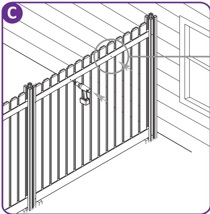
C - Place two 1.25 inch screws into the middle of the top rail
