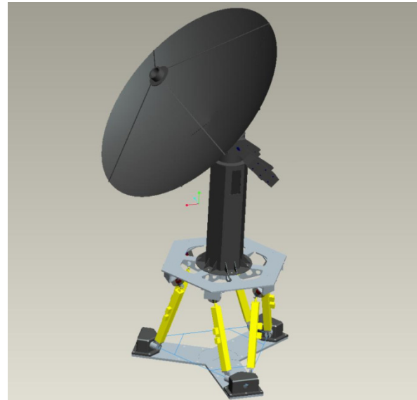
Figure 4: The Stewart platform with asymmetric load (45° degree of elevation).
