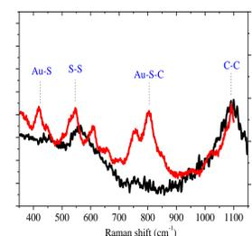
Raman Spectroscopy is an effective tool for detecting the presence of chemical bonds. Shown to the left is the normalized intensity Raman spectra of the bare corona (black) and the NOHM product (red). The characteristic Au-S, S-S and Au-S-C vibrations are indicated. This confirms that our corona has attached to the core.
