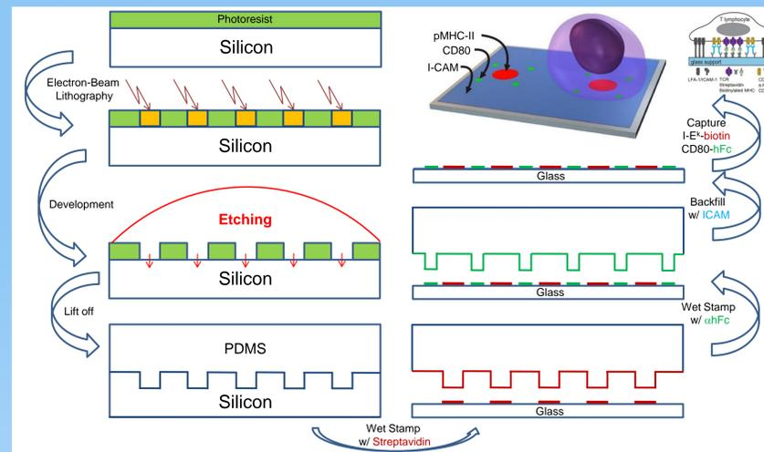
Figure 4: Master templates fabrication and sequential rounds of microcontact imprinting
