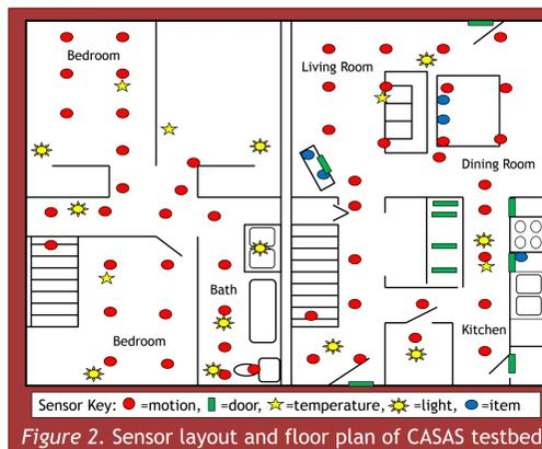
Figure 2. Sensor layout and floor plan of CASAS testbed
