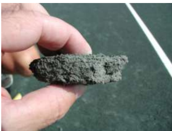
Picture 17 shows ideal surface thickness of 1"
