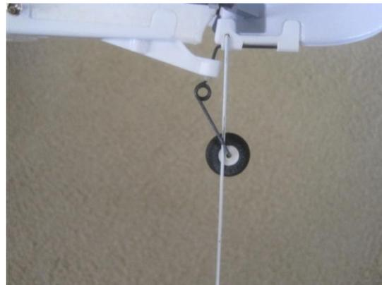
View the assembly from above and ensure the rudder shaft and paddle are in alignment with the flying rudder as it appears in the photo below. Cut off excess rudder shaft beyond the collar as desired. See photo next page.
