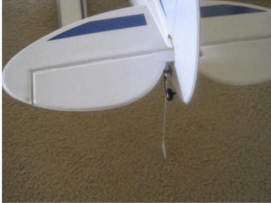
When transporting the aircraft, a small screw (not provided), placed on the left side fuselage in the plastic tail wheel bracket, can hold the water rudder out of the way as shown in photo below.
