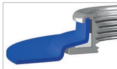
*All Tri-Sure<sup>®</sup> G2 and G3/4 4s<sup>®</sup> flanges are designed for maximum performance in combination with the Tri-Sure<sup>®</sup> R-Plug<sup>™</sup>.*
