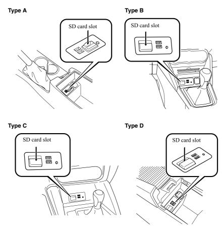
When inserting the SD card, never move the slider on the side of the SD card to the LOCK position. If the slider is set to LOCK, the SD card cannot be read and the navigation system will not operate.
