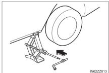
and raise the vehicle high enough so that the spare tire can be installed. Before removing the lug nuts, make sure your Toyota is firmly in position and that it cannot slip or move.
