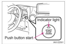
7 Press the push button start after both the KEY indicator light (green) in the combination meter and the push button start indicator light (green) illuminate.
