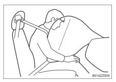
In addition, the front passenger air bag is designed to only deploy when the front passenger occupant classification sensor detects a passenger sitting on the front passenger's seat. For details, refer to the front passenger occupant classification system ( $\rightarrow$ P. 78).
