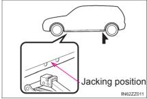
G Continue raising the jack head gradually by rotating the screw with your hand until the jack head is inserted into the jack-up position.
