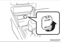
To prevent discharging of the battery, do not use the socket for long periods with the engine off or idling.
