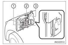
If it is at or near L, add enough coolant to the coolant reservoir to provide freezing and corrosion protection and to bring the level to F.
