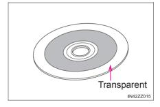
A new CD may have rough edges on its inner and outer perimeters. If a disc with rough edges is used, proper setting will not be possible and the CD player will not play the CD. In addition, the disc may not eject resulting in a malfunction.
