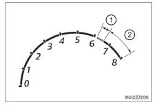
When the tachometer needle enters the STRIPED ZONE, this indicates to the driver that the gears should be shifted before entering the RED ZONE.
