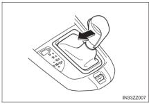
To return to automatic shift mode, shift the lever from M to D.
