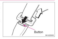
If a belt does not fully retract, inspect it for kinks and twists. If it is still not retracting properly, have it inspected at your Toyota dealer.
