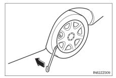
2 Loosen the lug nuts by turning them counterclockwise one turn each, but do not remove any lug nuts until the tire has been raised off the ground.
