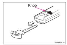
2 Twist a tape-wrapped flathead screwdriver in the direction of the arrow and open the cover slightly.
