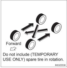
Inspect the tires for uneven wear and damage. Abnormal wear is usually caused by one or a combination of the following:
