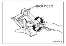
Place the jack under the jackup position closest to the tire being changed with the jack head squarely under the jackup point.
