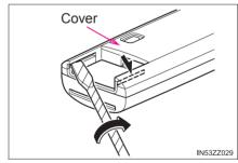
Insert the tape-wrapped flathead screwdriver into the gap and slide it in the direction of the arrow.
