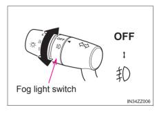
The fog lights will turn off when the headlights are set at high beams.
