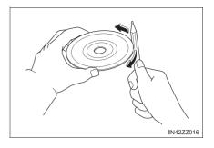
Remove the rough edges in advance by using a ball-point pen or pencil as shown below. To remove the rough edges, rub the side of the pen or pencil against the inner and outer perimeter of the CD.
