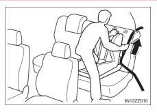
Inspect this function before each use of the child-restraint system. You should not be able to pull the shoulder belt out of the retractor while the system is in the automatic locking mode. When you remove the childrestraint system, be sure the belt fully retracts to return the system to emergency locking mode before occupants use the seat belts.
