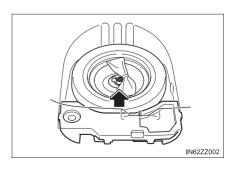
3 Turn the wing bolt and jack screw counterclockwise.
