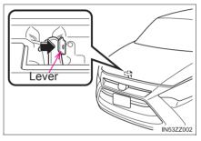
3 Grasp the support rod in the padded area and secure it in the support rod hole indicated by the arrow to hold the hood open.
