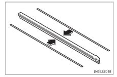
4 Carefully insert the new blade rubber. Then install the blade assembly in the reverse order of removal.
