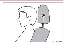
To raise a head restraint, pull it up to the desired position.
