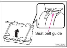
Press the seatback rearward and lock it in place. After returning the seatback to its upright position, make sure it is securely locked.
