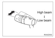
When the headlight high-beams are on, the headlight high-beam indicator light is turned on.
