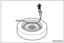
13 Pass the belt through the buckle, then pull the belt end to secure the flat tire.
