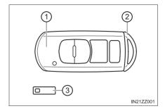
To use the auxiliary key, press the knob and pull out the key (smart key).
