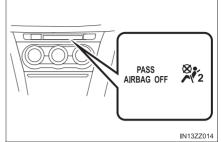
If the front passenger occupant classification sensor is normal, the indicator light turns on when the ignition is switched ON. The light turns off after a few seconds. Then, the indicator light turns on or is off under the following conditions:
