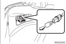
5 Install the new bulb in the reverse order of the removal procedure.
