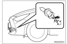
5 Turn the socket and bulb assembly to remove it. Carefully remove the bulb from its socket in the reflector by gently pulling it straight backward out of the socket.
