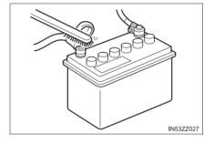
If the vehicle will not be used for an extended time, disconnect the battery cables and charge the battery every six weeks.
