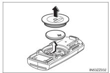
6 Insert a new battery with the positive pole facing up, and then cover the battery with the battery cap.
