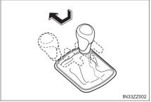
If shifting to R is difficult, shift back into neutral, release the clutch pedal, and try again.
