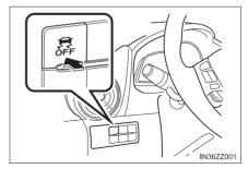
Press the switch again to turn the TCS/DSC back on. The DSC OFF indicator light will turn off.
