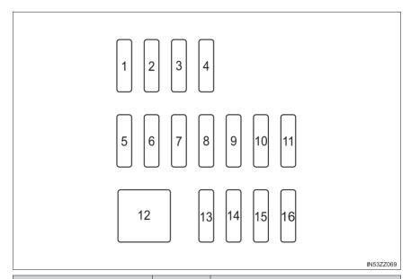
FUSE PROTECTED COMPONENT **DESCRIPTION RATING** 1 2 3 4 Accessory sockets 5 F.OUTLET 15 A 6 7 AT IND AT shift indicator (if equipped) 7.5 A 8 MIRROR 7.5 A Power control mirror 9 10 P.WINDOW2 25 A Power windows 11 R.WIPER 15 A 12 13 SRS2/ESCL 14 15 A Seat warmer (if equipped) 15 **SEAT WARM** 20 A
