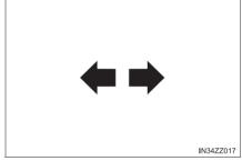
Depress the hazard warning flasher and all the turn signals will flash. The hazard warning indicator lights in the instrument cluster flash simultaneously.
