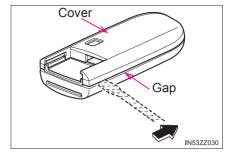
4 Twist the flathead screwdriver in the direction of the arrow and remove the cover.
