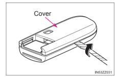
5 Remove the battery cap, then remove the battery.
