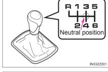
Your vehicle is equipped with a device to prevent shifting to R (reverse) by mistake. Push the shift lever downward and shift to R
