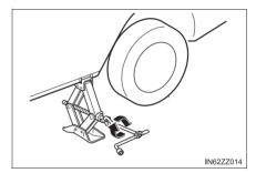
9 Remove the lug nuts by turning them counterclockwise; then remove the wheel and center cap.
