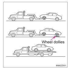
When towing with the rear wheels on the ground, release the parking brake.
