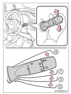
Washer/wiper dual operation The wiper will automatically operate a couple of times after the washer squirts.
