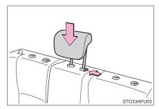
5 Pull the seatback lock release knob and fold the seatback down.
