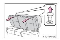
2 Align the head restraint with installation holes and push it down to the lock position.
