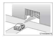
When the vehicle is hit by water, snow, dust, etc. from a vehicle ahead
