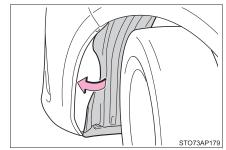
11 Attach the fender liner retainer.
