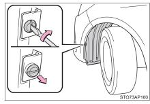
Partly remove the fender liner until the light bulb is visible.
