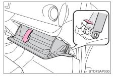
Push in each side of the glove box to disconnect the upper claws.
