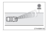
When the vehicle is being parked in a place where there is a low hanging object at the height of the front sensor
