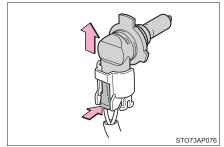
Replace the light bulb, plug the connector, and then install the bulb base.
