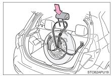
8 Hold the buckle and pull the belt to secure the tire.
