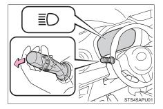
2 Press the Automatic High Beam switch.
