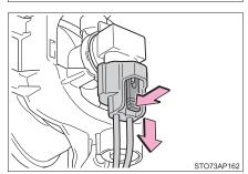
6 Turn the bulb base counterclockwise and remove.
