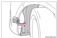
5 Unplug the connector while pressing the lock release.
