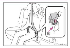
2 To release the hooked plate "A", insert the plate "B", the key into the hole on the buckle.
