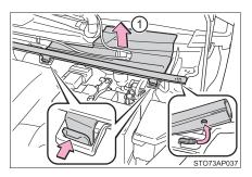
Remove the battery terminal cover and then the fuse box cover.
