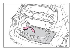
Remove the spare wheel cushion (if equipped), then loosen the center fastener that secures the spare tire.
