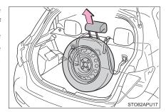
6 Pass the belt through the center hole of the flat tire wheel.
