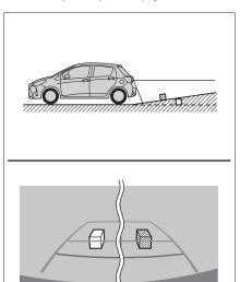
When the ground behind the vehicle slopes down sharply
