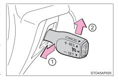
Resuming is available when the vehicle speed is more than approximately 25 mph (40 km/h).
