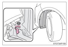
Remove the fender liner retainer.
