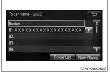
When an MP3/WMA/AAC disc or USB memory device is being used, the folder can be selected. When a Bluetooth<sup>®</sup> device or iPod is being used, the album can be selected.
