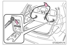
5 Lay the flat tire on the luggage floor so that the outer side of the tire wheel faces toward the rear of the vehicle. Detach the rear center head restraint from the seat and release the belt.
