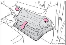
4 Pull out the glove box and disconnect the lower claws.
