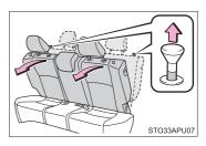
2 Pull the head restraint up while pushing the lock release button.
