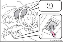
5 Wait for a few minutes with the engine switch in the "ON" position and then turn the engine switch to the "LOCK" position.
