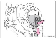
5 Turn the bulb base counterclockwise and remove.
