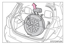
6 Pass the belt through the center hole of the flat tire wheel.
