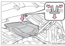
Partly remove the fender liner.
