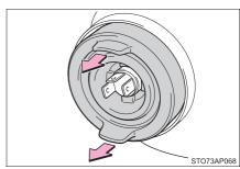
Release the bulb retaining spring.
