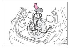
8 Hold the buckle and pull the belt to secure the tire.
