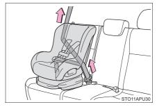
If the child restraint has a top tether strap, the top tether strap should be latched onto the top tether strap anchor. (→P. 63)
