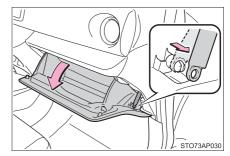
3 Push in each side of the glove box to disconnect the upper claws.
