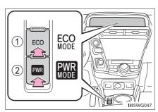
When the "ECO" switch is pressed, the "ECO MODE" indicator comes on in the instrument cluster.
