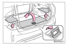
2 Fold inwards together with the head restraint installation hooks and secure. Then, stow in the auxiliary boxes.
