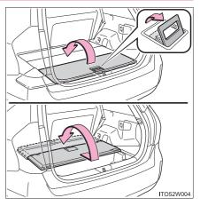
2 Remove the left side deck board and then remove the center auxiliary boxes.
