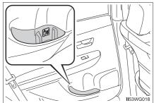
The type B cup holder on the center console (front side): The cup holder can be used store small objects if the inner tray is removed.
