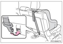
3 Outboard only: Adjust the head restraint to the downmost position while pressing the lock release button.
