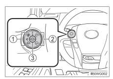
Cursor switch (CD, MP3/WMA disc, Bluetooth®, iPod or USB mode)
