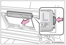
4 Slide and pull out the filter. Replace it with a new one.
