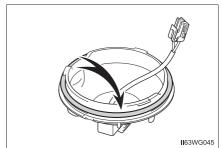
5 Replace the light bulb, and set the connector.
