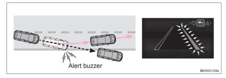
When the system judges that the vehicle is deviating from the current traffic lane, an alert buzzer sounds and it prompts cautions from the display screen of the multi-information display.
