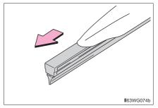
Install the 2 metal plates from the removed wiper rubber to the replacement wiper rubber.
