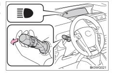
2 Press the Automatic High Beam switch.
