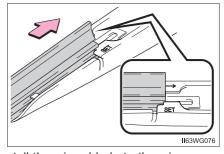
After installing the wiper rubber, install the wiper blade to the wiper arm and secure the stopper.
