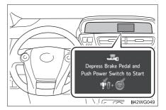
3 Press the power switch shortly and firmly.
