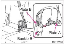
3 Put plates A and B on top of each other and insert them into the holder.
