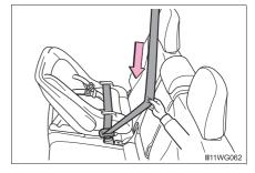
The straint system down into the rear seat, allow the shoulder belt to retract until the child restraint system is securely in place.
