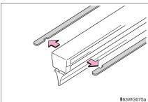
When installing, insert the wiper rubber in the direction opposite that used during the removal procedure until the wiper rubber becomes locked and stops moving.
