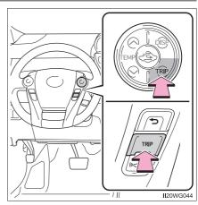
The function can be reset by pressing the TRIP button for longer than 1 second when the average fuel consumption is displayed on the trip meter.
