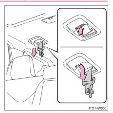
2 Connect by inserting plate B into buckle B until a click sound is heard.
