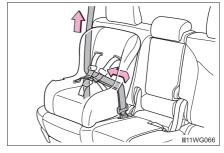
If the child restraint has a top tether strap, the top tether strap should be latched onto the top tether strap anchor.  $(\rightarrow P. 70)$
