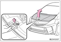
3 Hold the hood open by inserting the supporting rod into the slot.
