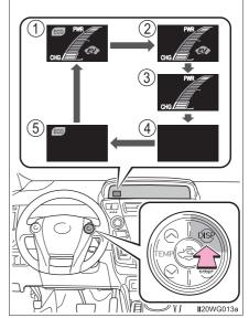
3 Press and hold the DISP button for 1 second or more to complete the setup.
