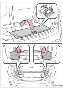
Lift the center deck board and then lift the side deck boards.
