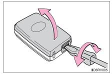
3 Remove the depleted battery.
