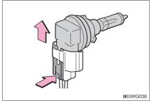
Replace the light bulb, and install the bulb base.
