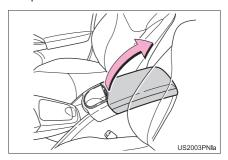
2 Open the cover and connect iPod using an iPod cable.
