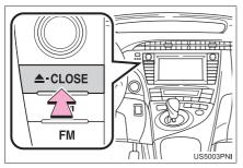
The display will slide down, opening the DVD slot. 2 Insert a disc into the disc slot.
