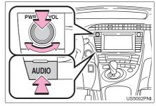
"AUDIO" button: Press to display screen buttons for the audio/video system (audio control mode).
