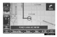
2 Touch "Preferences" to display conditions that can be selected when the system determines the route to the destination.
