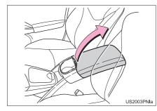
3 Open the cover and connect iPod using an iPod cable.
