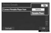
"Vehicle": Touch to connect the audio system to the portable player.
