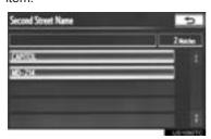
When the desired item is selected, the "Confirm Destination" screen may be displayed. If "Go" is touched on the "Confirm Destination" screen, the navigation system performs a search for the route. (See "STARTING ROUTE GUIDANCE" on page 76.)
