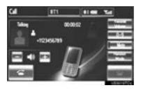
To adjust the volume of the other party's voice: Touch "-" or "+", turn the "PWR VOL" knob, or use the volume switch on the steering wheel.
