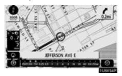
Touch or lost to change the scale of the map display. The scale bar and indicator at the bottom of the screen indicates the map scale menu. The scale range is 150 feet (50 m) to 250 miles (400 km).
