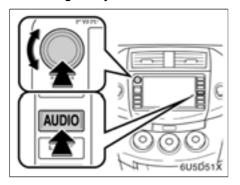
"AUDIO": Push this button to display touch screen buttons for audio system (audio control mode).
