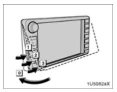
Adjustment of the angle of the display can be done by touching "TILT". Each touch "TILT" will tilt the display to positions 1, 2, 3 and then back to 0 in the reverse order.
