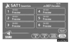
To scan the currently selected channel category: Touch "TYPE SCAN" briefly. "SCAN" appears on the display. The radio will find the next channel in the same channel category, stay there for a few seconds, and then scan again. To select a channel, touch "TYPE SCAN" a second time.
