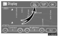
To display the screen in the day mode even with the headlight switch on, touch "Day Mode" on the adjustment screen for brightness and contrast control.
