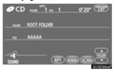
Push the "AUDIO" button and touch a MP3/WMA disc number to display this screen.
