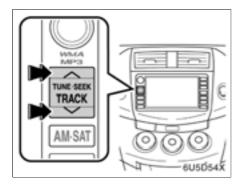
Push "∧" or "∨" sides of the "TUNE·SEEK/TRACK" button to step up or step down the station band.
