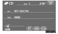
The function buttons for radio and CD player operation are displayed on the screen when the audio control mode is selected.
