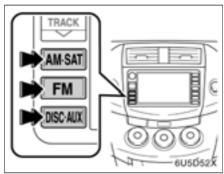
Push "AM·SAT", "FM" or "DISC·AUX" button to turn on the desired mode. The selected mode turns on immediately.
