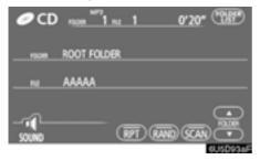
While the disc is playing, touch "SCAN" and hold it until the "FLD.SCAN" appears on the screen.
