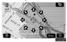
When an arrow facing the desired point is touched, the map scrolls in that direction. Releasing the finger from the arrow will stop the scrolling.
