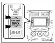
"TUNE-SEEK/TRACK" button: Use for a direct access to a desired track.
