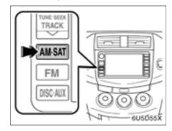
Push the "AM·SAT" button to choose either an AM station or a SAT (satellite) channel.
