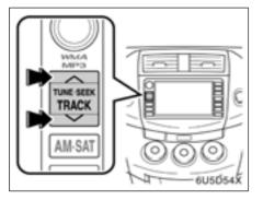
"TUNE-SEEK/TRACK" button: Use for direct access to a desired file.
