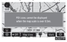
This message appears when the system is in the POI mode and the map scale is over 0.5 miles (800 m).
