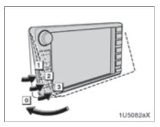
Adjustment of the angle of the display can be done by touching "TILT". Each touch "TILT" will tilt the display to positions 1, 2, 3 and then back to 1 in the reverse order.
