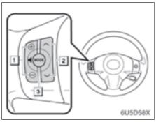
Some parts of the audio system can be adjusted with the switches on the steering wheel.
