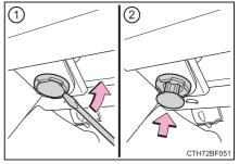
Securely attach cables or chains to the towing eyelet.
