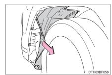
4 Unplug the connector while depressing the lock release.
