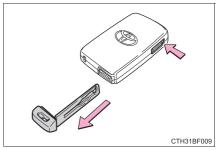
After using the mechanical key, store it in the electronic key. Carry the mechanical key together with the electronic key. If the electronic key battery is depleted or the entry function does not operate properly, you will need the mechanical key.  $(\rightarrow P. 510)$
