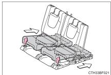
3 Pull the lever to unlock the seatback and then fold the seatback down.
