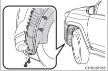
3 Partly remove the fender liner.
