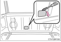
2 Tear the plastic film. Remove the cover.
