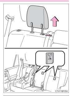
2 Open the anchor bracket cover, latch the hook onto the anchor bracket and tighten the top tether strap.
