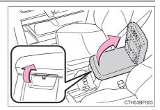
■The separator can be used in either of the positions shown in the illustration
