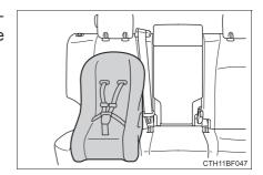
2 Run the seat belt through the child restraint system and insert the plate into the buckle. Make sure that the belt is not twisted.
