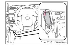
Remove the fuse with the pullout tool.
