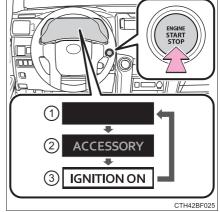
\*: If the shift lever is in a position other than P when turning off the engine, the engine switch will be turned to ACCESSORY mode, not to off.
