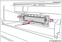
4 Remove the air conditioning filter and replace it with a new one.
