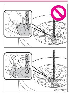
Vehicles with kinetic dynamic suspension: While raising, pull the tire towards the rear of the vehicle, taking care that the tire goes up without catching on any surrounding part to prevent it from flying forward during a collision or sudden braking.
