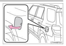
2 Turn the fuel tank cap slowly to open. Hang the fuel tank cap on the back of the fuel filler door.
