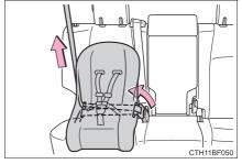
5 If the child restraint has a top tether strap, the top tether strap should be latched onto the top tether strap anchor. (→P. 66)
