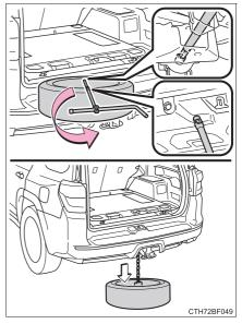
Pull out the spare tire and remove the holding bracket.
