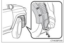
3 Partly remove the fender liner.
