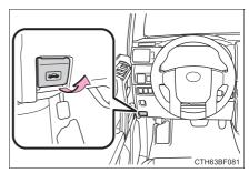
2 Push the auxiliary catch lever to the left and lift the hood.
