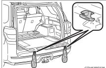
Type B only: To use the grocery bag hooks, slide the slide deck to the full-slide locked position.
