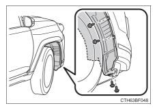
Partly remove the fender liner.
