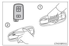
(2) Touch the lock sensor (the indentation on the upper part of the door handle) to lock the doors.
