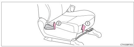
1 Seat position adjustment lever Seatback angle adjustment lever
