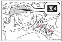
The initial shift range in S mode is set automatically to "4" according to vehicle speed. However, the initial shift range may be set to "3" if Al-SHIFT has operated while the shift lever was in the D position.  $(\rightarrow P. 220)$
