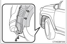
3 Partly remove the fender liner.
