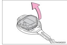
Open the case cover using a coin protected with tape etc. and remove the depleted battery.
