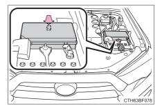
Driver's side instrument panel Remove the lid.
