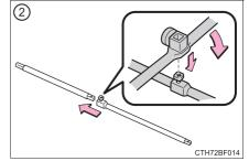
3 Assemble the jack handle and the jack handle extension bar and tighten the screw.
