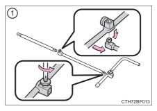
2 Assemble the jack handle extension bars and tighten the bolt.
