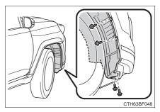
3 Partly remove the fender liner.
