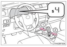
The initial shift range in S mode is set automatically to "4" according to vehicle speed. However, the initial shift range may be set to "3" if Al-SHIFT has operated while the shift lever was in the D position.  $(\rightarrow P. 203)$
