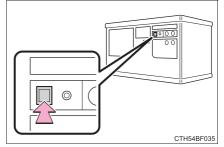
3 Press and hold the programmed HomeLink® button (located inside the vehicle) for 2 seconds and release it. Repeat this sequence (press/hold/release) up to 3 times to complete programming.
