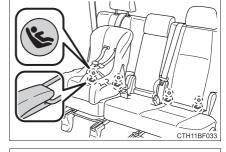
Seat belts equipped with a child restraint locking mechanism (ALR/ELR belts except driver's seat belt) (→P. 31)
