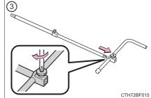
Insert the end of the jack handle extension into the lowering screw and turn it counterclockwise.
