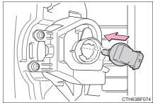
7 Turn clockwise and secure the bulb base.
