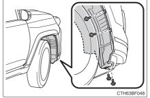
3 Partly remove the fender liner.
