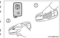
2 Touch the lock sensor (the indentation on the upper part of the door handle) to lock the doors.
