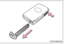
After using the mechanical key, store it in the electronic key. Carry the mechanical key together with the electronic key. If the electronic key battery is depleted or the entry function does not operate properly, you will need the mechanical key.  $(\rightarrow P. 451)$
