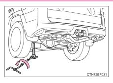
4 Firmly tighten each wheel nut two or three times in the order shown in the illustration.
