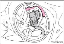
3 Unplug the connector while pulling the lock release.
