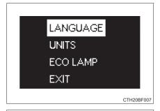
3 Press the "DISP" switch to select the desired setting, and then press and hold the "DISP" switch.
