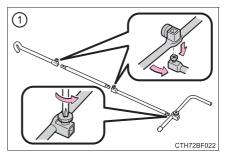
② Assemble the jack handle extension bars and the jack handle bar and tighten the bolts.
