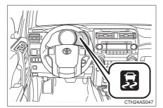
If all wheels spin, the slip indicator flashes to indicate that the active traction control system has been engaged.
