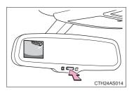
When the screen is displayed, press the "AUTO" button on the inside rear view mirror to switch the screen on/off.
