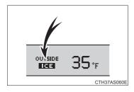
If the outside temperature lowers to 37 °F (3 °C) or below when the engine switch is in the "ON" position, the "ICE" indicator will come on to warn the driver that roads may be icy. Check the road surface and drive carefully. (The indicator will go off when the outside temperature rises to 41 °F [5 °C].)
