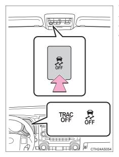
To turn the TRAC and VSC systems off, press and hold the button for more than 3 seconds while the vehicle is stopped.
