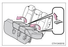
Swing the bottom cushions up by pulling the lock release strap.
