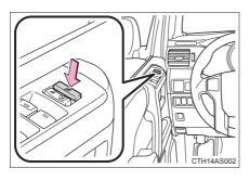
Press the switch down to lock the passenger window switches and back window switch.
