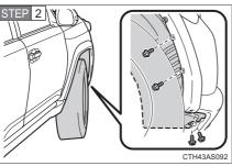
Remove the fender liner screws.
