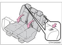
Push the lock release button and fold down the seatbacks.
