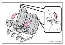
Pull the seatback lock release lever and fold the seatback down.
