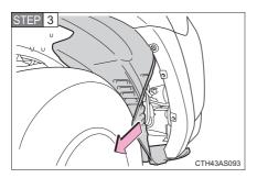
Partly remove the fender liner.
