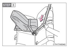
Fully extend the shoulder belt and allow it to retract to put it in lock mode. In lock mode, the belt cannot be extended.
