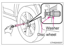
When replacing an aluminum wheel with an aluminum wheel, tighten the wheel nuts until the washers comes into contact with the disc wheel.
