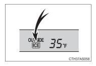
If the outside temperature lowers to 37 °F (3 °C) or below when the engine switch is in the "ON" position (vehicles without a smart key system) or the "ENGINE START STOP" switch is in IGNITION ON mode (vehicles with a smart key system), the "ICE" indicator will come on to warn the driver that roads may be icy. Check the road surface and drive carefully. (The indicator will go off when the outside temperature rises to 41 °F [5 °C].)
