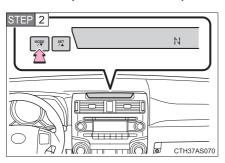
In deviation calibration mode  $(\rightarrow P.~447)$ , press and hold the "MODE/ $\blacktriangledown$ " button to change to circling calibration mode.
