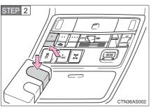
Press and hold one of the HomeLink® buttons and the transmitter button. When the HomeLink® indicator light changes from a slow to a rapid flash after 20 seconds, release both buttons.
