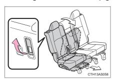
Lift the lever on the back of the seatback and fold down the seat-back. The seat will slide forward.
