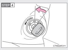
Vehicles without a smart key system: Stop the engine by turning the engine switch to "ACC".
