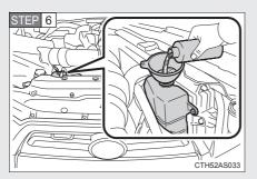
Add engine coolant if necessary.
