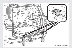
To use the grocery bag hooks, slide the slide deck to the full-slide locked position.  $(\rightarrow P. 454)$
