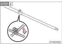
When connecting the jack handle extensions, use the jack handle to tighten the square head bolt. Make sure that the bolt fits into the depression on the joint.
