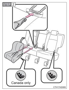
Latch the hooks of the lower straps onto the LATCH anchors. If the child restraint has a top tether strap, the top tether strap should be latched onto the top tether strap anchor.
