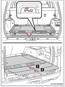
Slide the deck while turning the lock release lever, and then release the lever after sliding the deck to the lock position.
