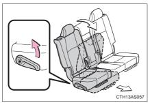
Pull up the lever and fold down the seatback. The seat will slide forward.
