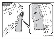
Partly remove the fender liner.
