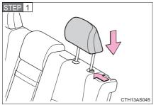
Adjust the head restraints to the downmost position.
