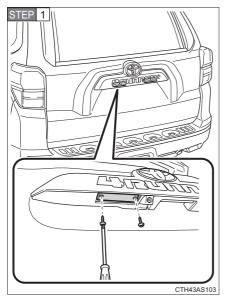
Remove the screws and lens.
