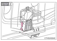
Tear the plastic film. Remove the cover.
