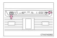
The hour or minute can be moved forward or backward by pressing the "MODE/ $\blacktriangledown$ " or "SET/ $\blacktriangle$ " button while pressing and holding the "H" or "M" button. If the "MODE/ $\blacktriangledown$ " or "SET/ $\blacktriangle$ " button is also pressed and held in the above operation, the hour or minute will move faster.
