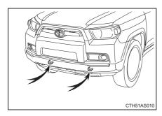
If a tow truck is not available in an emergency, your vehicle may be temporarily towed using a cable or chain secured to the emergency towing eyelet(s). This should only be attempted on hard surfaced roads for short distances at low speeds.
