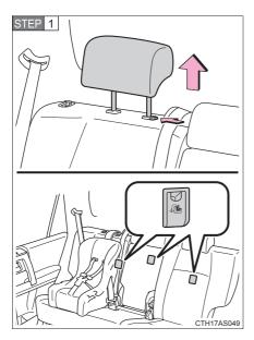
Secure the child restraint system using a seat belt or the lower anchors, and remove the head restraint.
