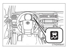
If the vehicle is in danger of slipping or rolling backward when starting on an incline, or if any of the drive wheels spins, the slip indicator flashes to indicate that the VSC/TRAC (TRC)/hill-start assist control systems are operating.
