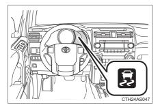
The slip indicator will flash to indicate that the downhill assist control system is operating, and the stop lights and high mounted stoplight will turn on.
