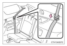
Pass the seat belts through the seat belt hangers and secure the seat belt plates.
