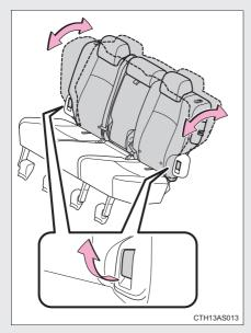
Pull up the seatback angle adjustment lever until the lock is released.
