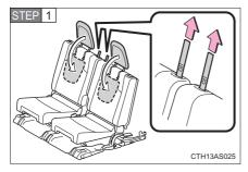
Pull the strap to fold down the head restraint.
