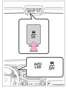
To turn the TRAC system off, quickly press and release the button.
