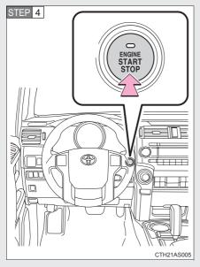
Press the "ENGINE START STOP" switch.
