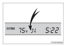
If "•" appears on the left side of the direction display, circling calibration needs to be performed.
