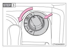
Push the "UNLOCK" button and turn the four-wheel drive control switch to H4L.
