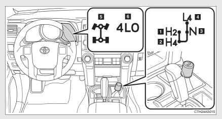
The four-wheel drive indicator comes on when H4, N or L4 mode is selected.
