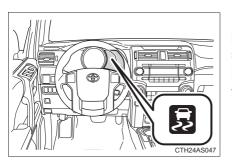
If the vehicle is in danger of slipping or if any of the drive wheels spins, the slip indicator flashes to indicate that the VSC/TRAC systems are operating.
