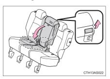
Pull the center seatback angle lever behind the seatback and fold the seatback down.
