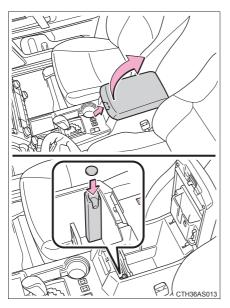
Lift the lid while pulling up the knob to release the lock.
