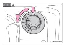
Push the "UNLOCK" button and then push and turn the fourwheel drive control switch to L4L.
