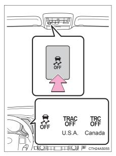
To turn the TRAC (TRC) and VSC systems off, press and hold the button for more than 3 seconds while the vehicle is stopped.
