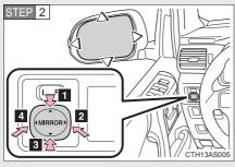
To adjust the mirror, press the switch.
