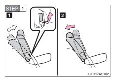
Fold the seatback while pulling the seatback angle adjustment lever. Return the seatback and secure it at the first lock position.  $(\rightarrow P. 63)$
