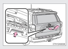
Raise the back door while pushing up the back door opener switch.
