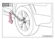
Slightly loosen the wheel nuts (one turn).
