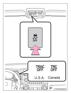
To turn the TRAC (TRC) system off, quickly press and release the button.
