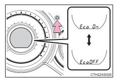
Eco Driving Indicator Light can be switched on or off by pressing and holding the display change button.
