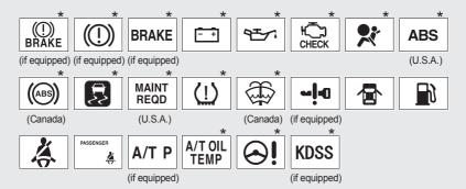
\*: These lights turn on when the "ENGINE START STOP" switch is turned to IGNITION ON mode (vehicles with a smart key system) or the engine switch is turned to the "ON" position (vehicles without a smart key system) to indicate that a system check is being performed. They will turn off after the engine is started, or after a few seconds. There may be a malfunction in a system if a light does not come on, or if the lights do not turn off. Have the vehicle inspected by your Toyota dealer.
