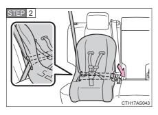
Run the seat belt through the child restraint system and insert the plate into the buckle. Make sure that the belt is not twisted.
