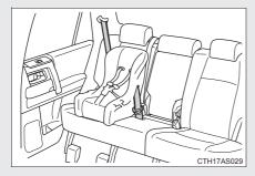
Seat belts equipped with a child restraint locking mechanism (ALR/ELR belts except driver's seat belt) (→P. 77)
