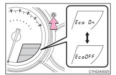
Eco Driving Indicator Light can be switched on or off by pressing and holding the display change button.
