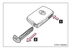
To take out the mechanical key, push the release button and take the key out.
