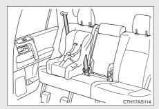
Seat belts equipped with a child restraint locking mechanism (ALR/ELR belts except driver's seat belt) (→P. 86)
