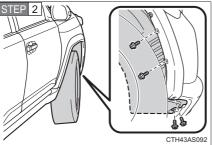
Remove the fender liner screws.
