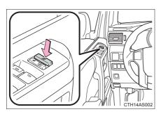
Press the switch down to lock the passenger window switches and back window switch.
