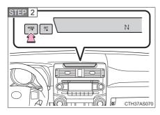
In deviation calibration mode  $(\rightarrow P. 482)$ , press and hold the "MODE/ $\blacktriangledown$ " button to change to circling calibration mode.
