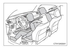
The pretensioner helps the seat belt to quickly restrain the occupant by retracting the seat belt when the vehicle is subjected to certain types of severe frontal and side collision or a vehicle rollover.
