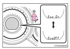
Eco Driving Indicator Light can be activated or deactivated by pressing and holding the display change button.
