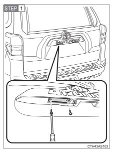
Remove the screws and lens.
