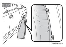
Turn the steering wheel in the opposite direction of the parking light and front side marker light that you wish to replace.
