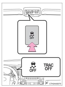
To turn the TRAC and VSC systems off, press and hold the switch for more than 3 seconds while the vehicle is stopped.
