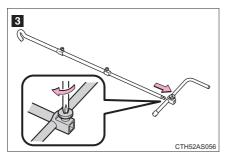
Assemble the jack handle extension bar and the jack handle and tighten the screw.
