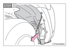
Partly remove the fender liner.
