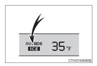
If the outside temperature lowers to 37°F (3°C) or below when the engine switch is in the "ON" position, the "ICE" indicator will come on to warn the driver that roads may be icy. Check the road surface and drive carefully. (The indicator will go off when the outside temperature rises to 41°F [5°C].)
