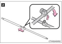
Assemble the jack handle extension bars and tighten the bolt.
