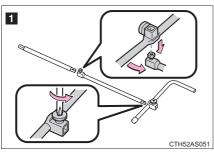
Loosen the bolt and the screw using either the jack handle or a screwdriver.
