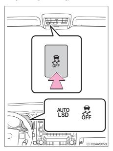
To turn the TRAC system off, quickly press and release the switch.
