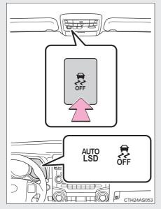
Press the VSC off switch to turn on the system.
