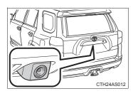
The rear view monitor system camera is located on the back door as shown in the illustration. The camera uses a special lens. The distance of the image that appears on the screen differs from the actual distance.
