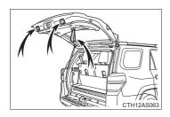
Lower the back door using the back door strap and/or the back door handle, and make sure to push the back door down from the outside to close it.
