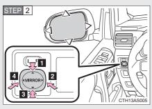
To adjust the mirror, press the switch.
