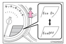
Eco Driving Indicator Light can be activated or deactivated by pressing and holding the display change button.
