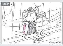
Tear the plastic film. Remove the cover.
