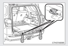
To use the grocery bag hooks, slide the slide deck to the full-slide locked position.
