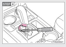
Pry the cover up with a flathead screwdriver or equivalent tool.
