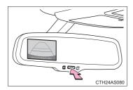
STEP 1 Push and hold the "AUTO" button for 6 to 12 seconds.
