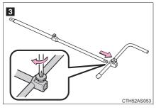
3 Assemble the jack handle and the jack handle extension bar and tighten the screw.
