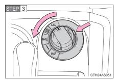
Push the "UNLOCK" button and turn the four-wheel drive control switch to H4L.
