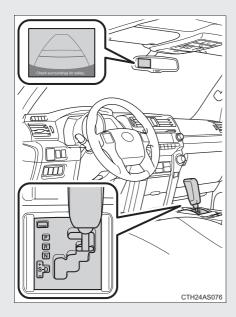
The rear view image is displayed when the shift lever is in R.
