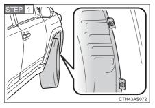
Turn the steering wheel in the opposite direction of the front turn signal light and daytime running light that you wish to replace.
