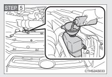
Add engine coolant if necessary.
