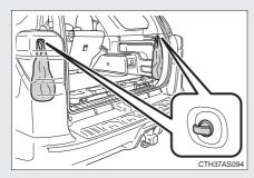
Slide the deck while turning the lock release lever, and then release the lever after sliding the deck to the lock position.
