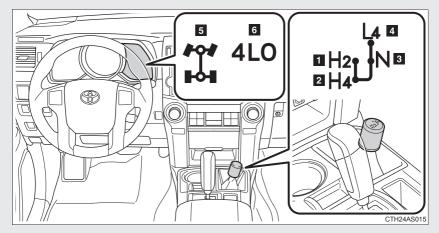
The four-wheel drive indicator comes on when H4, N or L4 mode is selected.
