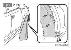
Partly remove the fender liner.
