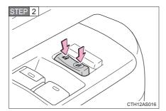
Shift the shift lever to P or N, and press and hold the driver's door lock switch ( or or or of or approximately 5 seconds and then release.
