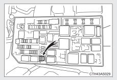
Only type A fuse can be removed using the pull-out tool.
