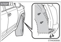
Partly remove the fender liner.
