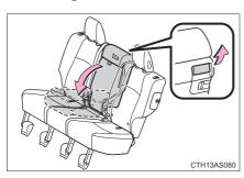
Pull the center seatback angle lever behind the seatback and fold the seatback down.
