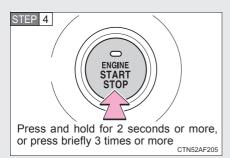
Vehicles with a smart key system: To stop the engine, press and hold the "ENGINE START STOP" switch for 2 consecutive seconds or more, or press it briefly 3 times or more in succession.
