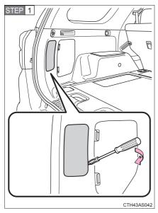
Open the back door and remove the cover.
