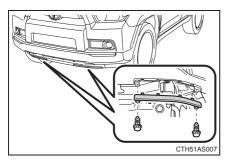
Vehicles with a front spoiler only: Before using the front emergency towing eyelet(s), remove the cover(s).
