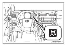
If the vehicle is in danger of slipping or if any of the drive wheels spins, the slip indicator flashes to indicate that the TRAC/VSC systems are operating.
