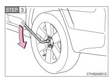
Slightly loosen the wheel nuts (one turn).
