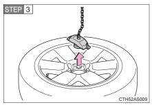
Pull out the spare tire and remove the holding bracket.
