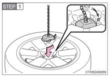
Lay down the tire with the outer side facing up, and install the holding bracket.
