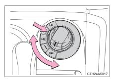
Push the "UNLOCK" button and turn the four-wheel drive control switch to H4L or H4F.
