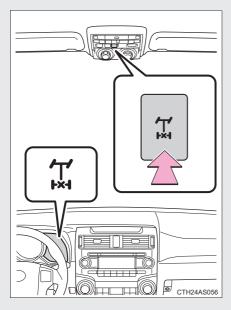
Press the switch to lock the rear differential.
