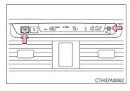
The hour or minute can be moved forward or backward by pressing the "MODE/ $\blacktriangledown$ " or "SET/ $\blacktriangle$ " button while pressing and holding the "H" or "M" button. If the "MODE/ $\blacktriangledown$ " or "SET/ $\blacktriangle$ " button is also pressed and held in the above operation, the hour or minute will move faster
