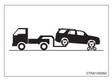
Full-time 4WD models: Use a towing dolly under the front wheels.
