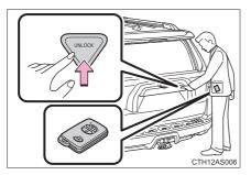
Press the button to unlock the door.
