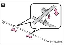
Assemble the jack handle extension bars and the jack handle bar and tighten the bolts.
