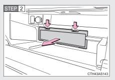
Open the glove box and remove the cover.
