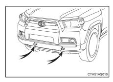
If a tow truck is not available in an emergency, your vehicle may be temporarily towed using a cable or chain secured to the emergency towing eyelet(s). This should only be attempted on hard surfaced roads for short distances at low speeds.
