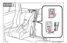
Open the anchor bracket cover, latch the hook onto the anchor bracket and tighten the top tether strap.
