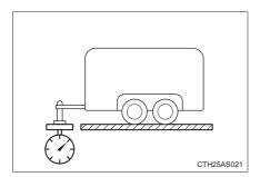
The load placed on the trailer hitch ball. ( $\rightarrow$ P. 301)
