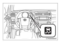
If the vehicle is in danger of slipping or rolling backward when starting on an incline, or if any of the drive wheels spins, the slip indicator flashes to indicate that the TRAC/VSC/hill-start assist control systems are operating.
