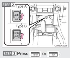
Open the cover and connect the portable audio device.
