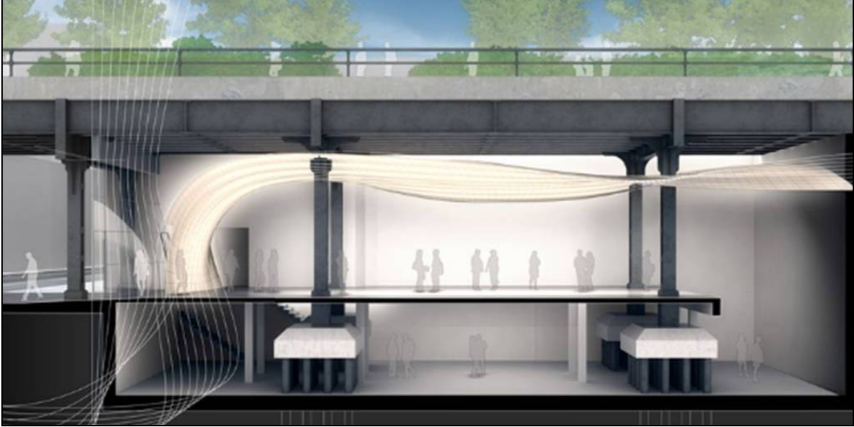
FIGURE 1 – RENDERING OF PTFE FABRIC AS SUSPENDED CEILING AND FAÇADE UNDERNEATH HISTORIC NEW YORK CITY WEST SIDE HIGHLINE (IMAGE BY: STUDIO MDA [1])
