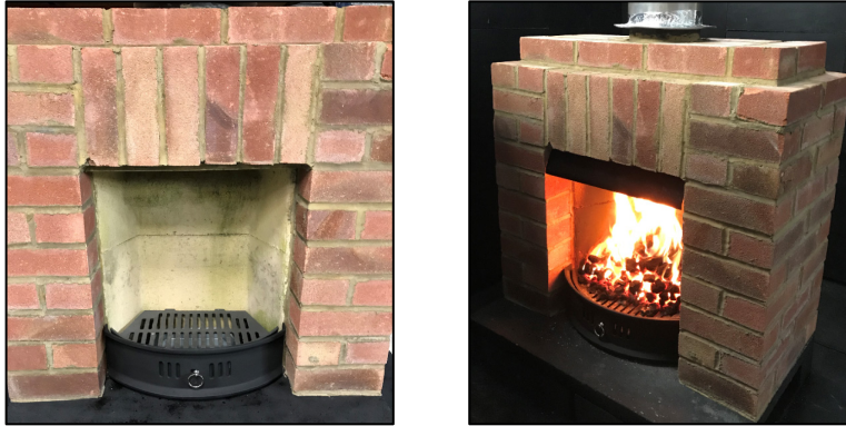
BSRIA Test open fireplace fitted with an 18" Solid Fuel Kit
