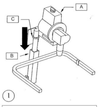
Insert the motor assembly (A) into the square tube of the foot (B) up to the stop ring (C).
