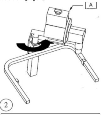
Rotate the motor assembly (A) to the right.
